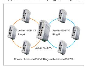
rings into a line or into multiple directions. In addition to extensibility, MultiRing TM has great diversity of various ring technologies. When MultiRing Menabled, JetNet 4508f V2 can connect RSR rings, TrunkRing Menabled a Super Ring together and simultaneously provide more Fast Ethernet Ring connectivities. This provides extensibility to new technologies while keeping the great backward compatibility.
